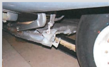
Damage to C-130: (top to bottom) Right wing; number four engine; flare dispenser hood; and gear door.
