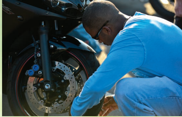
MSgt Danell Hall, Special Operations Central Command intelligence superintendent, checks tire pressure and wear patterns before MacDill AFB's CDS joint operations check ride.
