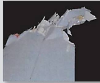
Damage to C-27: (left to right) Vertical stabilizer; Right wing tip.
