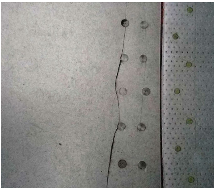
Engine inlet crack
