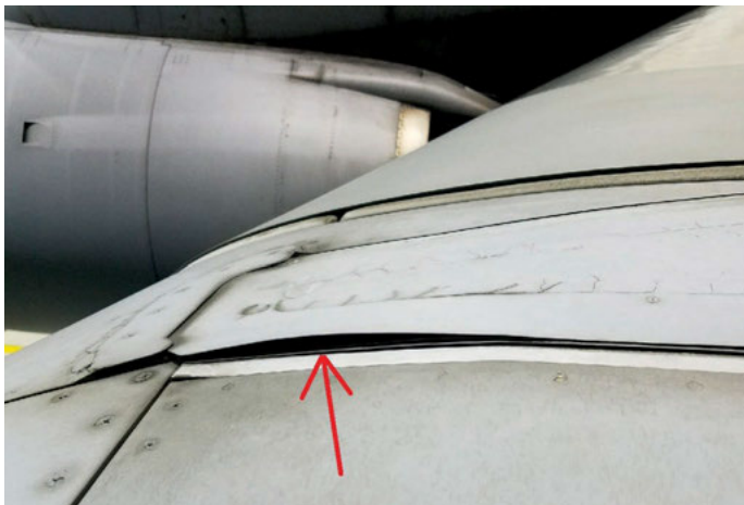
Right upper wing trapezoid panel delamination
