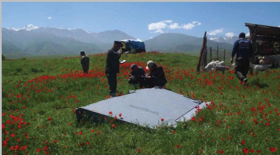
*Section of rudder as found north northeast of main debris field.*
