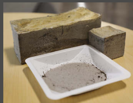
Biocement bricks made from soil obtained from a test range.
