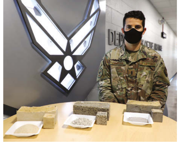
1Lt Alexander Compean with biocement samples produced by the AFRL team from a range of different starting materials. The team was able to make these bricks in two days without any high temperature processing.
