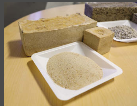
Biocement bricks made from commercial play sand.
