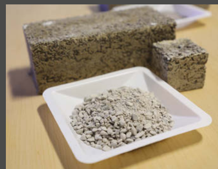
Biocement bricks made from commercial paver base.
