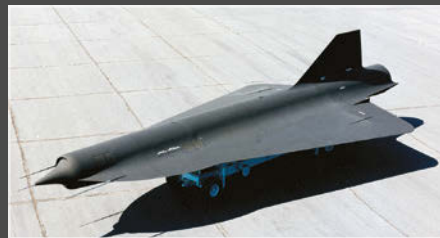
1962 Lockheed D-21, guided by an inertial navigation system on a preprogrammed path.
